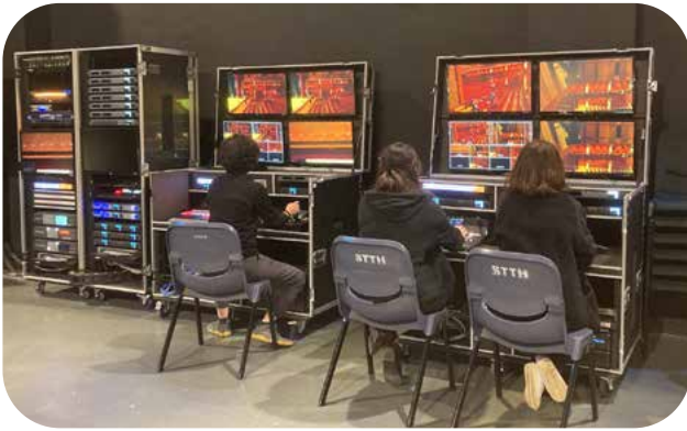
A live streaming system with user tie-line points has been installed in the Auditorium of the Sha Tin Town Hall, reflecting the trend for presenting programmes online.
